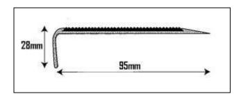
AS4 stair nosing has been designed for use on hard surfaces and is also suitable for vinyl and commercial style carpets. The nosing is fitted with PVC or anti-slip carborundum inserts. This profile can also be installed with a photo-luminescent insert.
